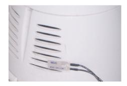
Figure 7. A piezo sensor attached to the rare engine grid of an electric blender.
