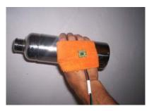
Figure 6. Accelerometer woven into a textile band.
